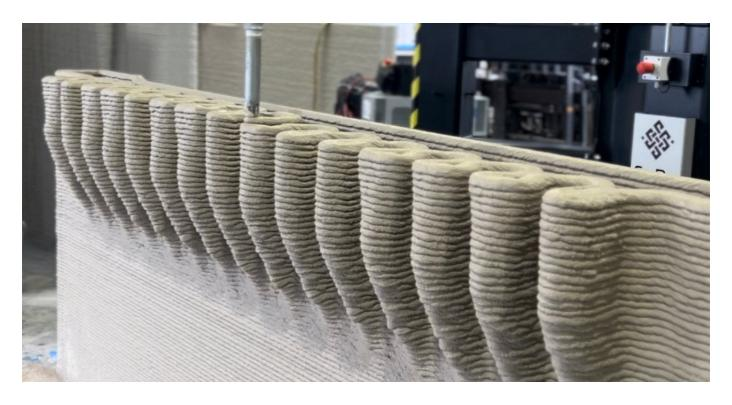
Kind Designs is 3D Printing the world's first Living Seawall slabs. The Living Seawall slabs are structurally identical to traditional seawall panels and can be used in any residential or commercial seawall project.
